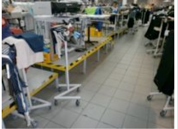
Cluster N° 8.2 Escape route markings on the floors are missing
